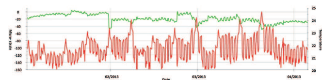
Figure 6: A typical variation pattern between the temperature (in red) and strain readings (in green) of sensor WT02 (i.e. sling wire JK) between January and April 2013.
