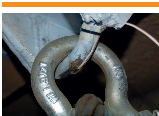
Figure 5: Resistance strain gauge, model FLA-3-11-3LT, on ceiling anchor.
