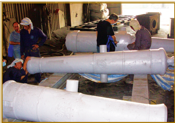
◆ Corrosion removal and coating application on the cannons
