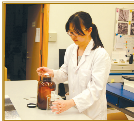
◆ A conservator preparing the gellan gum rigid gel
