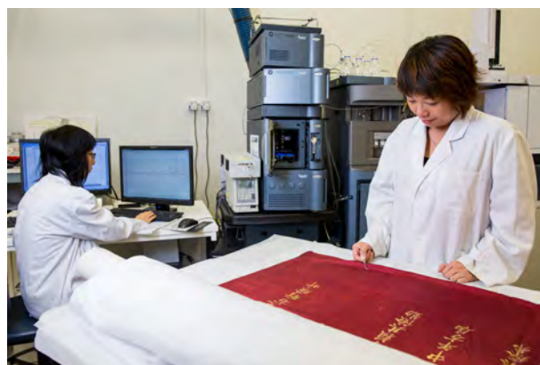
▲ Conservators analysing the dye with liquid chromatography equipped with time of flight mass spectrometer
