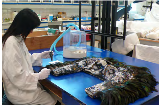
▲ A conservator reshaping the distorted peacock feather couture with an ultrasonic humidifier
