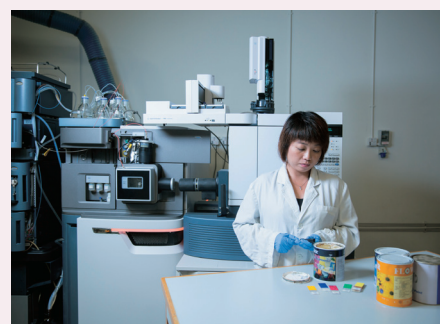
▲ A conservator preparing samples of interior paints for volatile emissions analysis by gas chromatography mass spectrometry
