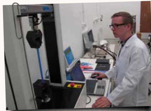
▲ Olli Petteri Peri conducting mechanical strength tests on synthetic polymers after accelerated ageing
