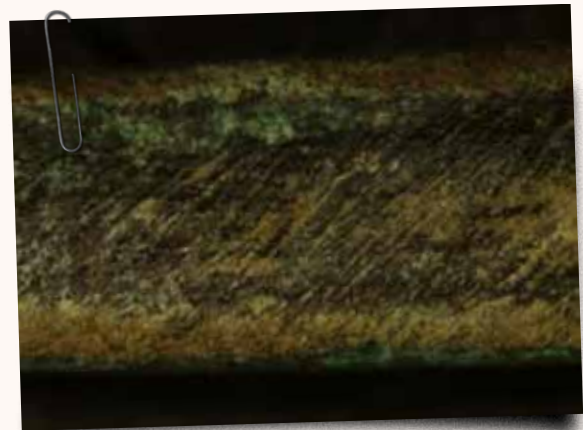
▲ The filing marks on a metal pin discovered under a microscope offer a clue about the early techniques of making bronze wares
